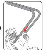
Using a screwdriver (not included) secure the legs using the two assembly screws provided, turn in a clockwise direction to tighten.
