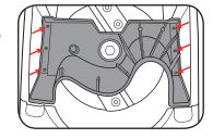
4. Place a screwdriver (not supplied) though the slot in the blade plate, this will secure the rotating blade plate in its position allowing you to remove both blades. The screws may be tight due to corrosion and dirt buildup. Ensure that the
