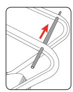
4. Place wheel spacer over protruding ends of axle.
