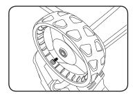
Insert a screwdriver through the holding hole on the axle and tighten the socket screws with hex key provided, turn in a clockwise direction.
